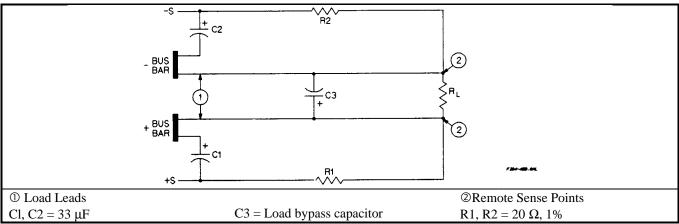
Figure 4-4b. Series 667xA Sense Lead Bypass Network
